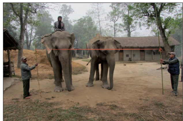
Figure 1. Trials with domestic elephant to establish correct fence height.
